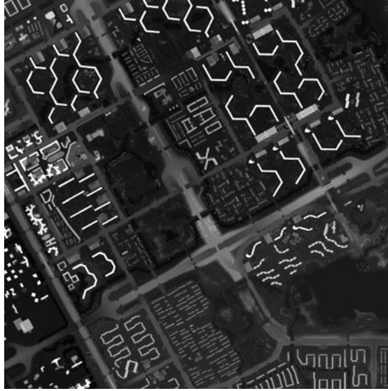
Figure 2.1: DSM from laser scanning of the study area in Amsterdam with 1 m resolution (with correction).
