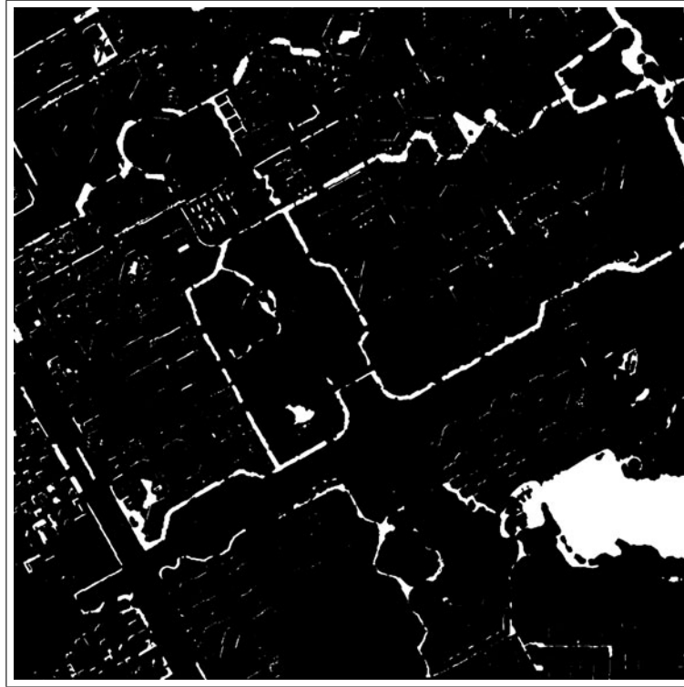
Figure 6.27: Water bodies after removal of objects that are masked by simulated shadow and buildings.
