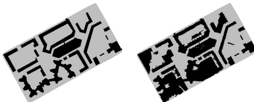
Figure 8.17: Buildings in a commercial area based on map (left) and extracted from image (right).
