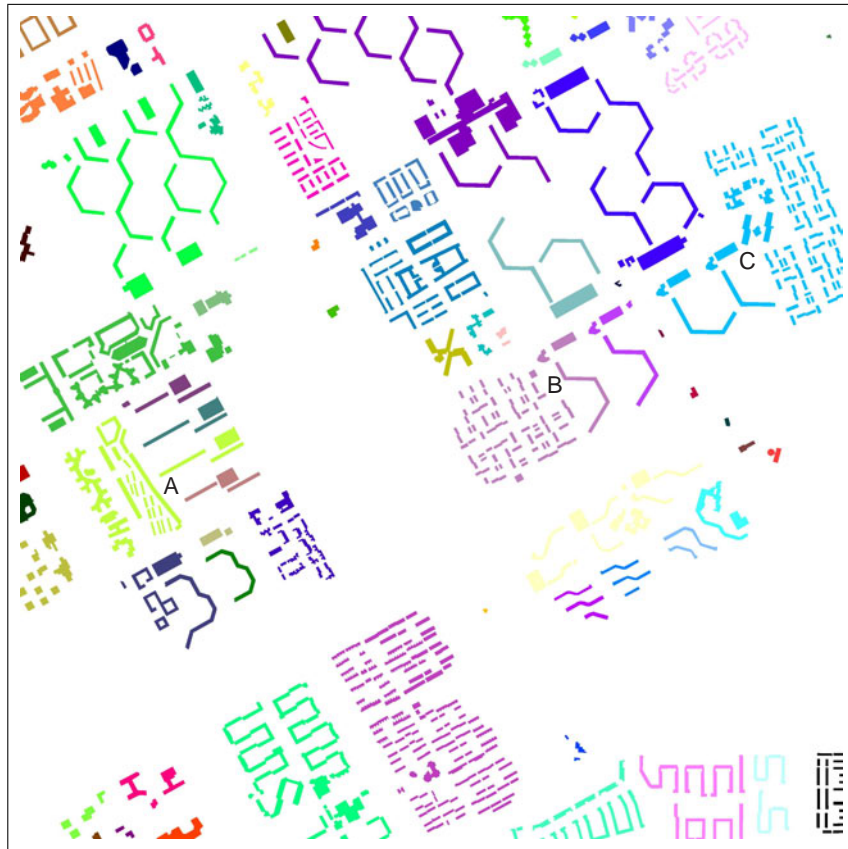
Figure 7.13: Clustered buildings where the shortest links are shorter than 40 m.
