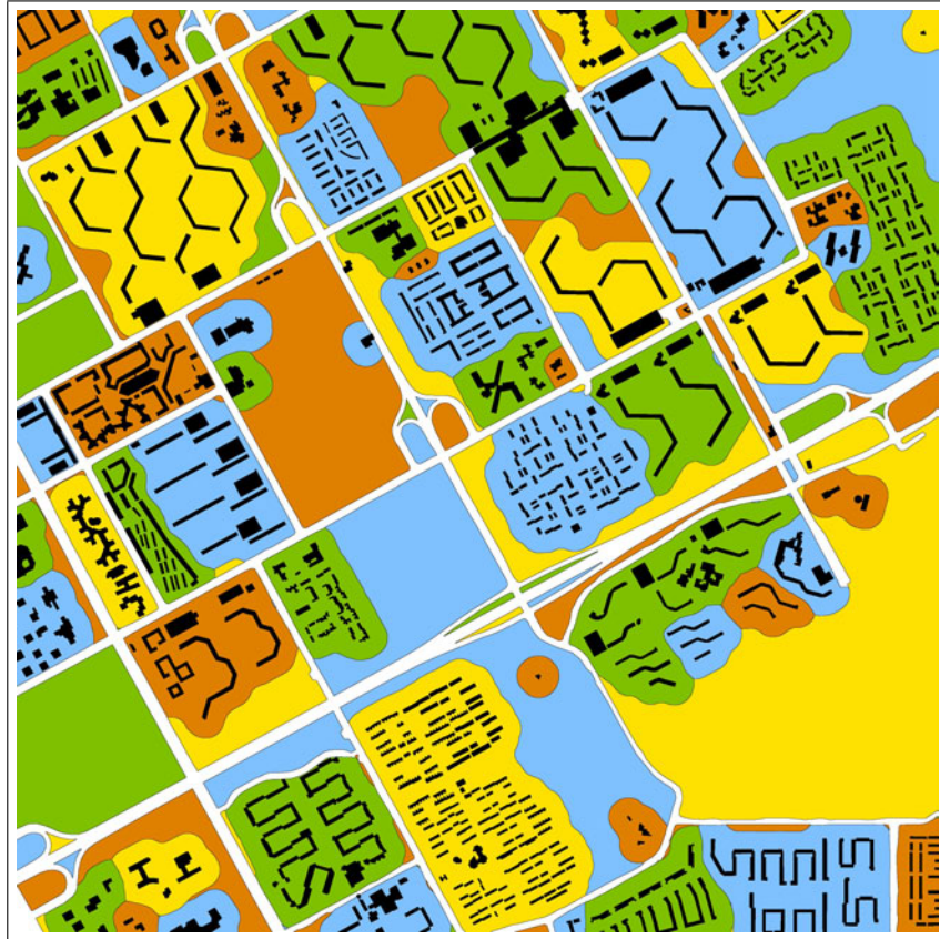
Figure 7.33: Spatial partitioning using the watershed algorithm based on the distance transformation and the road network (superimposed on all buildings).
