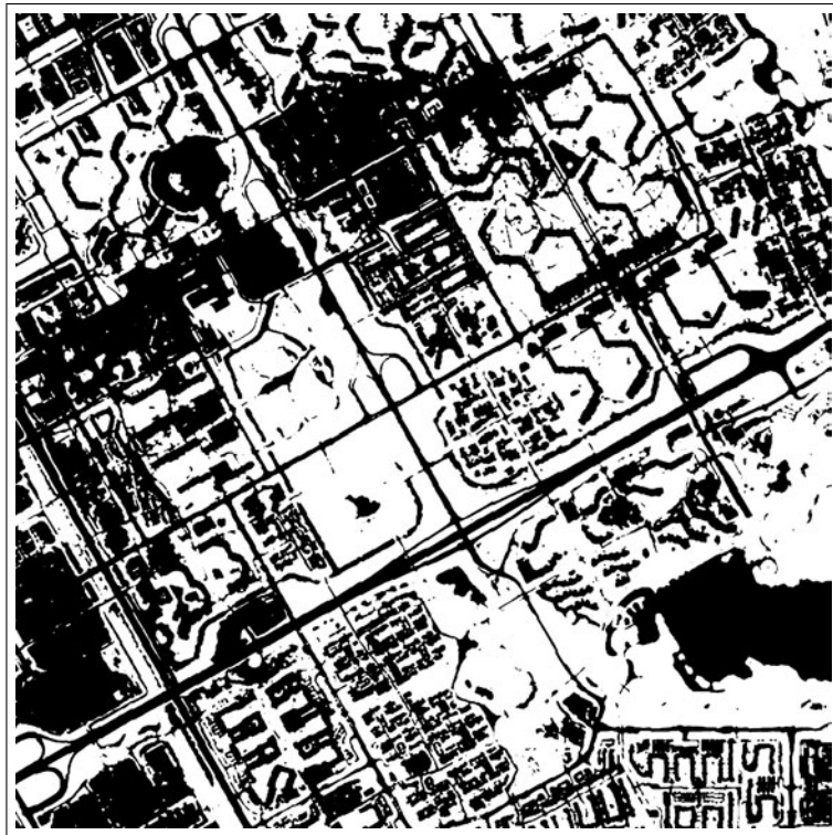
Figure 6.20: Green space extracted based on NDVI using fuzzy membership function.
