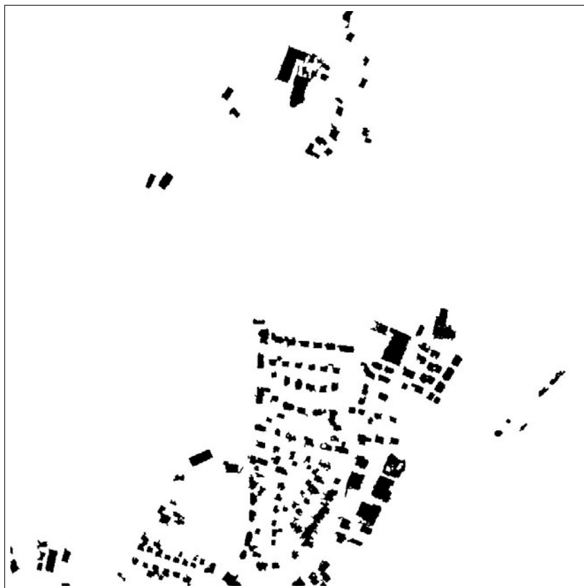
Figure 6.13: Buildings extracted by using 50 % as threshold for checking the size differences and using fuzzy membership functions based on other features, Ravensburg, Germany.
