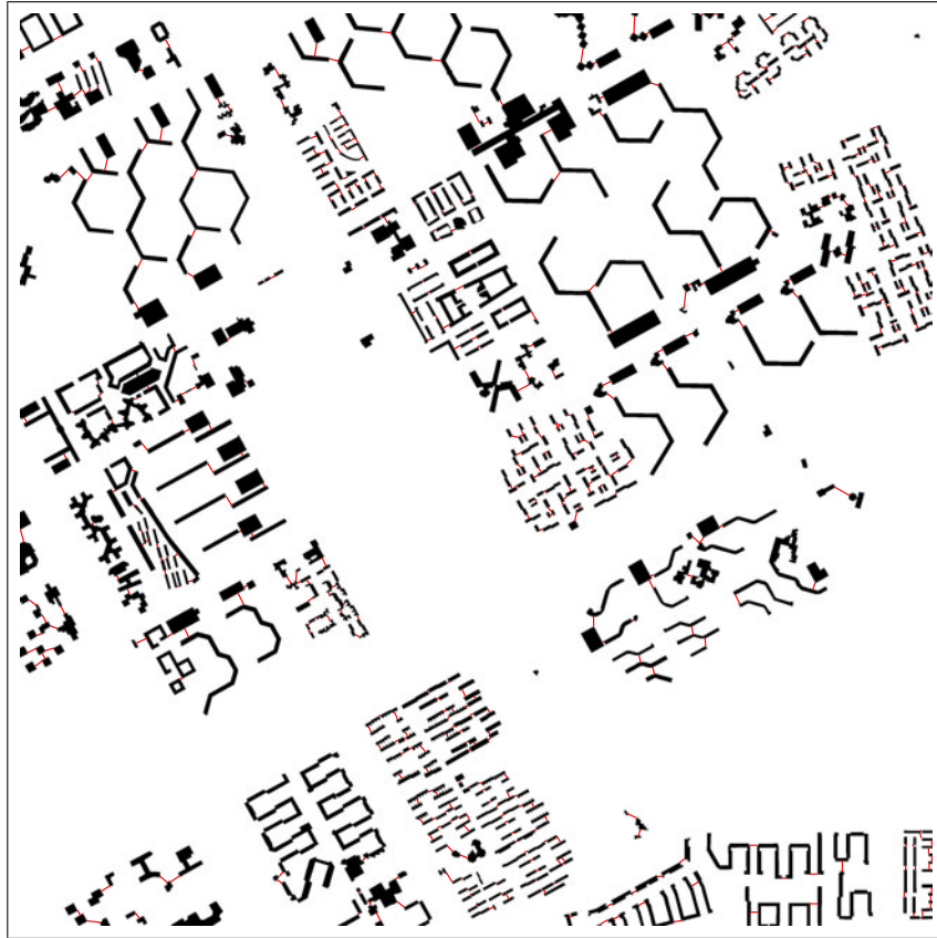
Figure 7.16: Linked buildings by the nearest neighbours closer than the threshold of 78.3 m.
