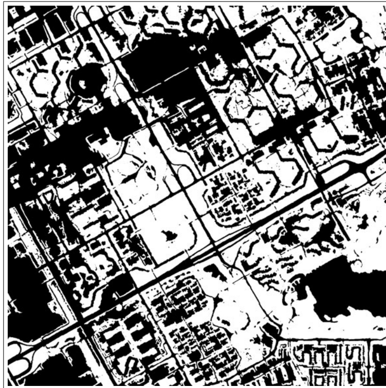
Figure 6.21: Green space after removal of objects smaller than 1000 m 2 .
